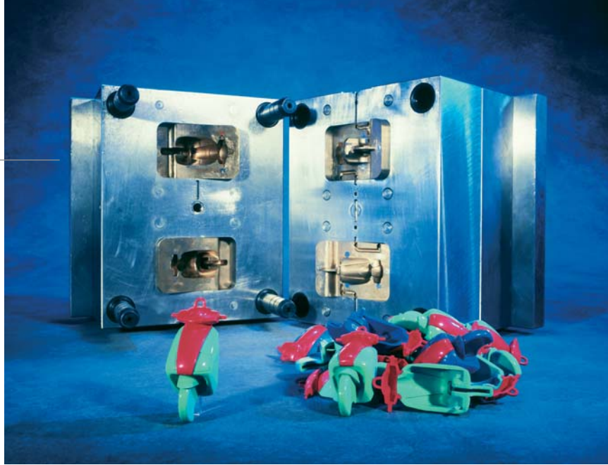
Twin coloured key ring, injection moulded with DirectTool.
